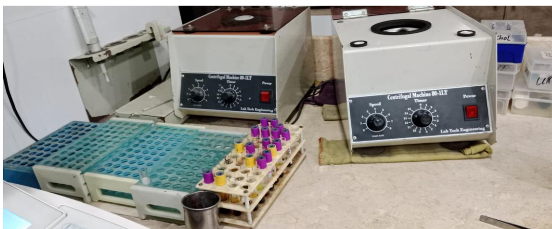
Figure 4. Blood sample preparation workflow for hematological and serological analysis, showing anticoagulant-treated and clotting tubes used for serum separation.
