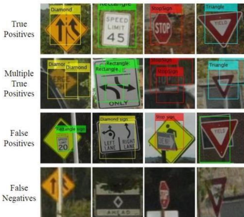
Figure 1 Illustration of True positives, false positives & false negatives using image based algorithm (Balali V. et al 2015)
