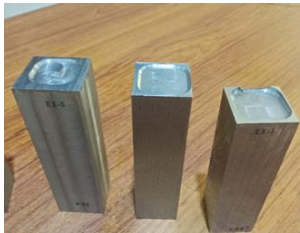
Figure 2. SS304 pocket specimens produced during the experimental trials.
